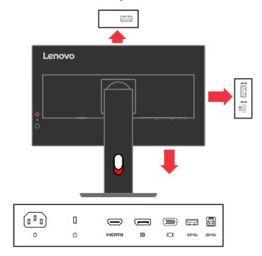
Connect one end of the DP cable to the DP connector on the back of the computer, and the other
