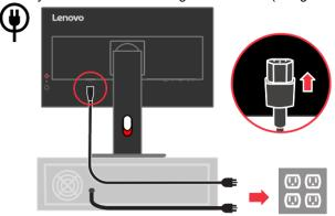
9. After attaching all necessary cables to your monitor and computer, organize all cables as shown below.
