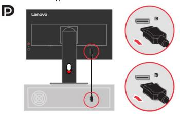
4. Connect one end of the HDMI cable to the HDMI connector on the back of the computer, and the other end to the HDMI connector on the monitor. Lenovo recommends that customers who require to use the HDMI input on their monitor purchase the "Lenovo HDMI to HDMI cable 0B47070".
