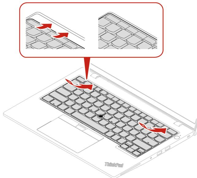
Step 3. Slightly press **1** and then slide the keyboard **2**. Ensure that the latches are secured under the keyboard frame.
