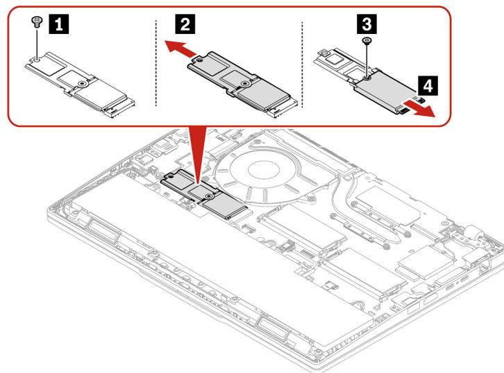
Step 2. Install the 2242 M.2 solid-state drive and its bracket in reverse order.
