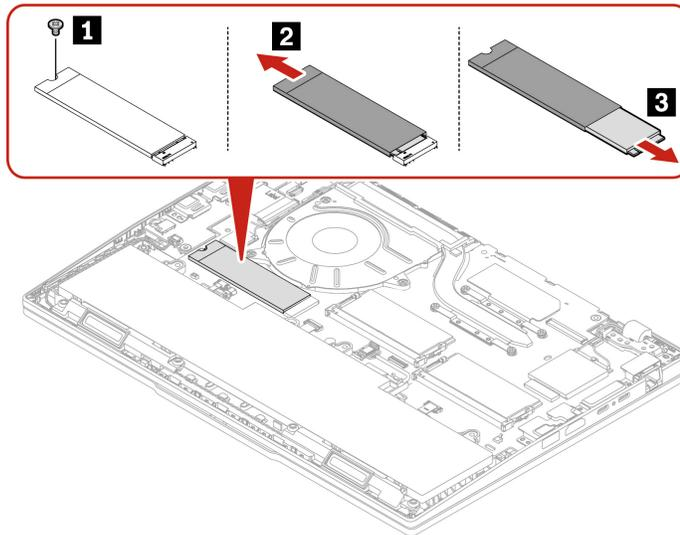
Step 2. Install the 2280 M.2 solid-state drive in reverse order.
