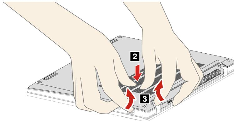
**Note:** Press the base cover assembly **2** with a pressure of less than 5 kg (11.02 lb). Release the pressure immediately when the base cover assembly is opened.
