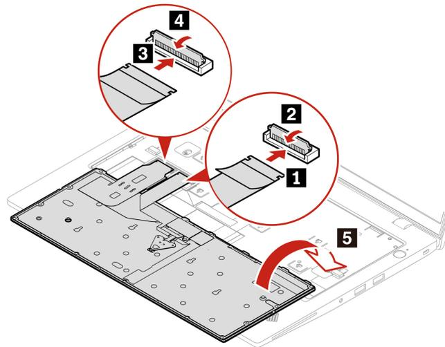
Step 2. Insert the keyboard into the keyboard bezel as shown. Ensure that the top edge of the keyboard (the edge that is close to the display) is under the keyboard bezel.
