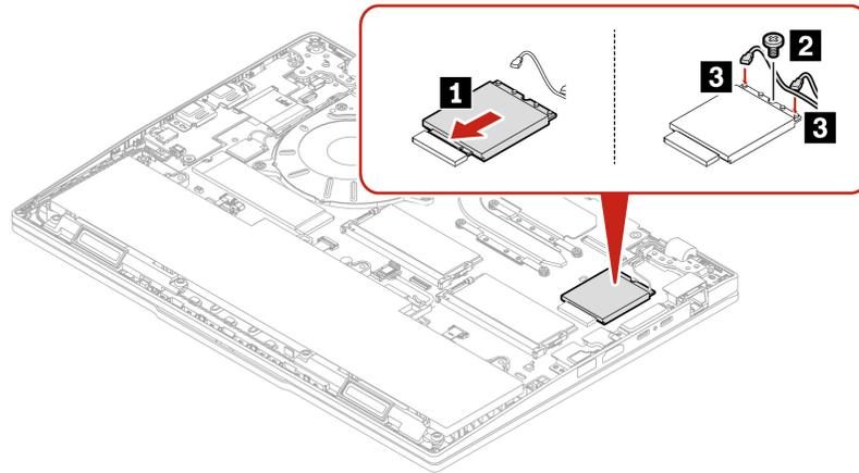
**Note:** When installing the wireless WAN card, ensure that you connect the orange cable to the connector labeled Orange on the card, and the blue cable to the connector labeled Blue.
