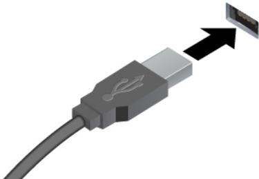
A grey USB-A connector cable with a standard rectangular plug and a black arrow pointing to the right. | <p>Connect USB-compatible devices, such as a USB keyboard, USB mouse, USB storage device, or USB printer.</p> <ul style="list-style-type: none"><li>• USB-A connector (Hi-Speed USB)</li><li>• USB-A connector (USB 5Gbps)</li><li>• USB-A connector (USB 10Gbps)</li></ul>
