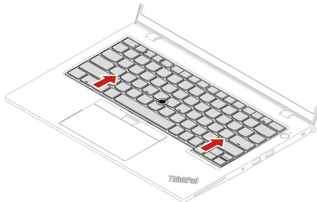
Step 3. Pivot the keyboard slightly upward **1** and then turn over the keyboard **2**.
