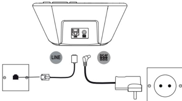
1. Plug the telephone line cord into the socket marked **LINE** on the rear of the base. Plug the other end of the telephone line cord into the telephone wall socket.
