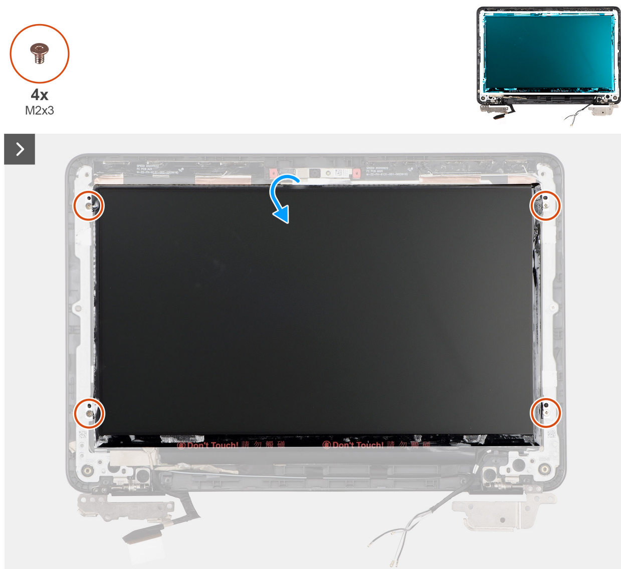
Figure 60. Removing the display panel
