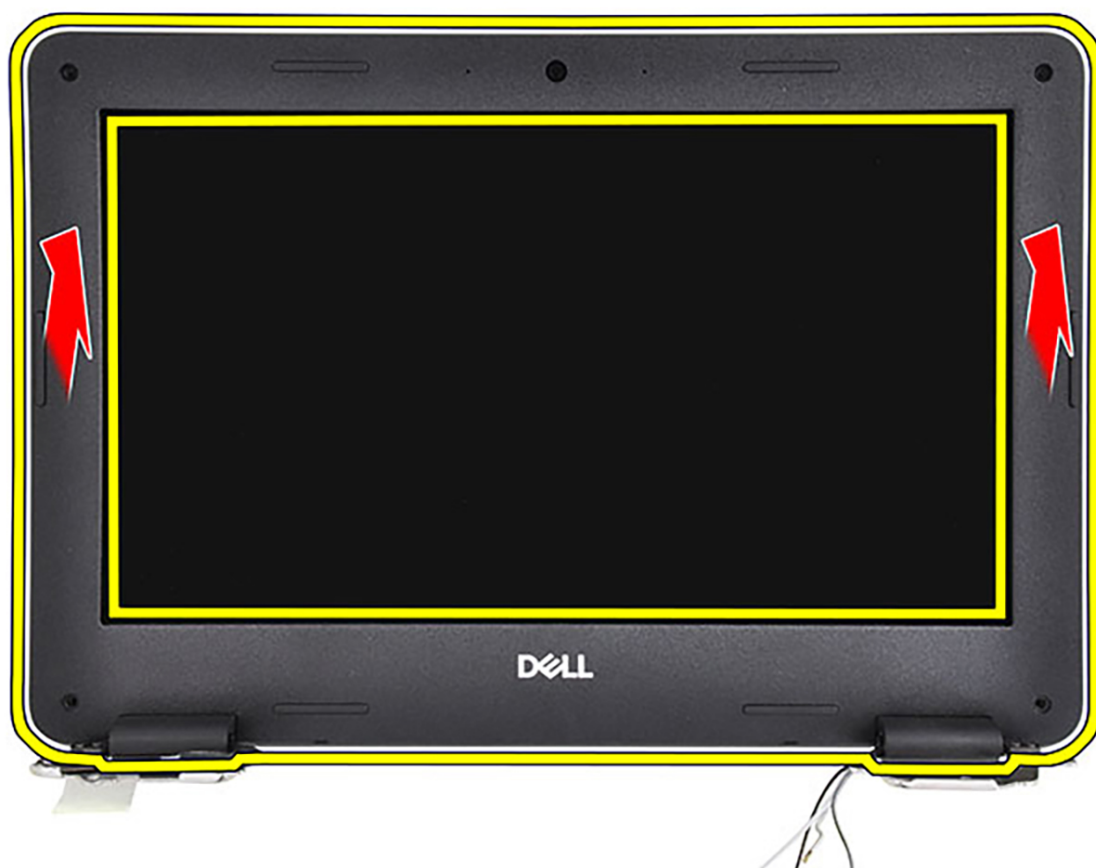
Figure 57. Remove the display bezel
