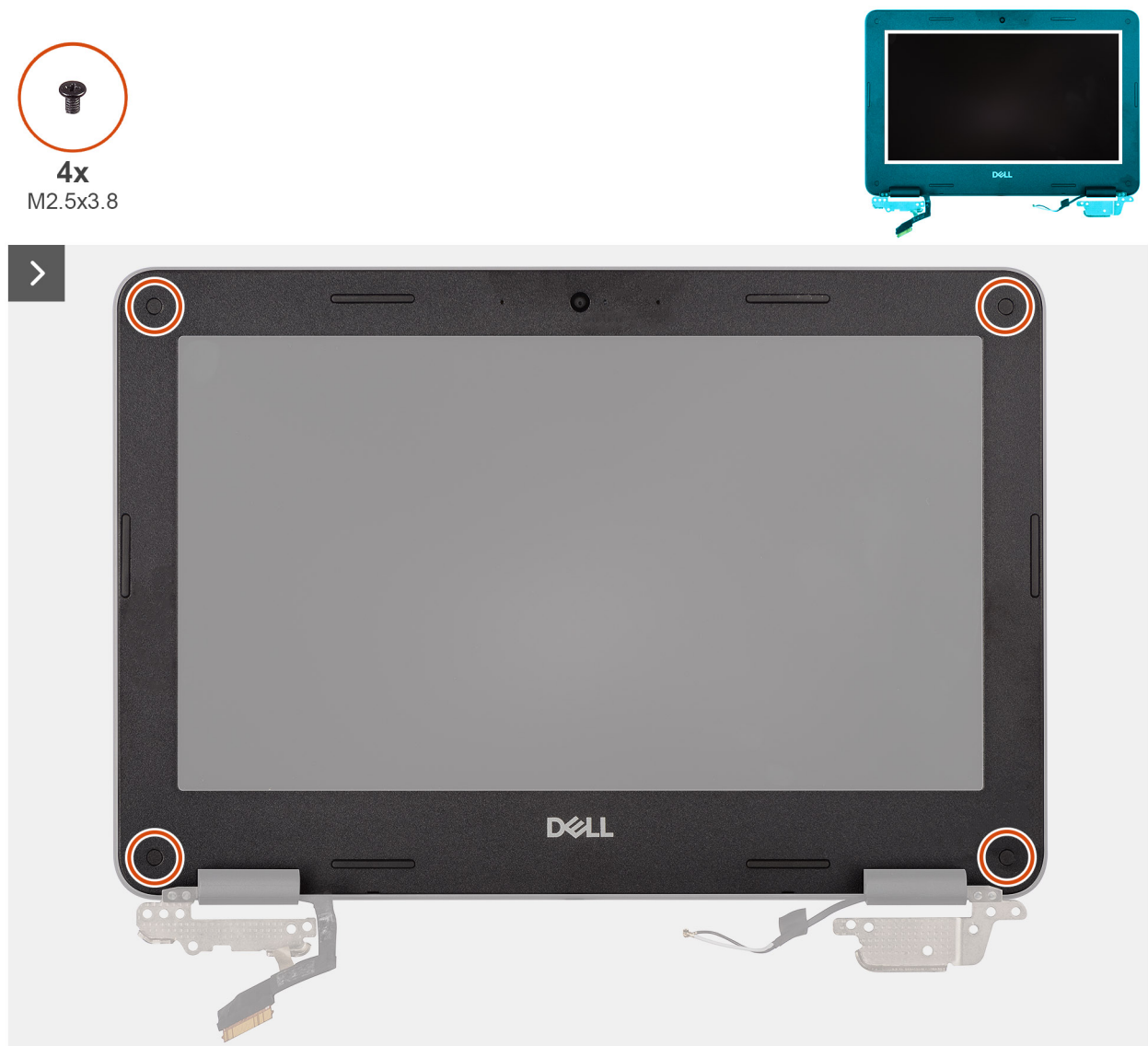
Figure 50. Removing the display bezel
