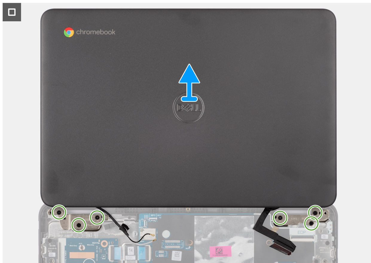
Figure 45. Removing the display assembly
