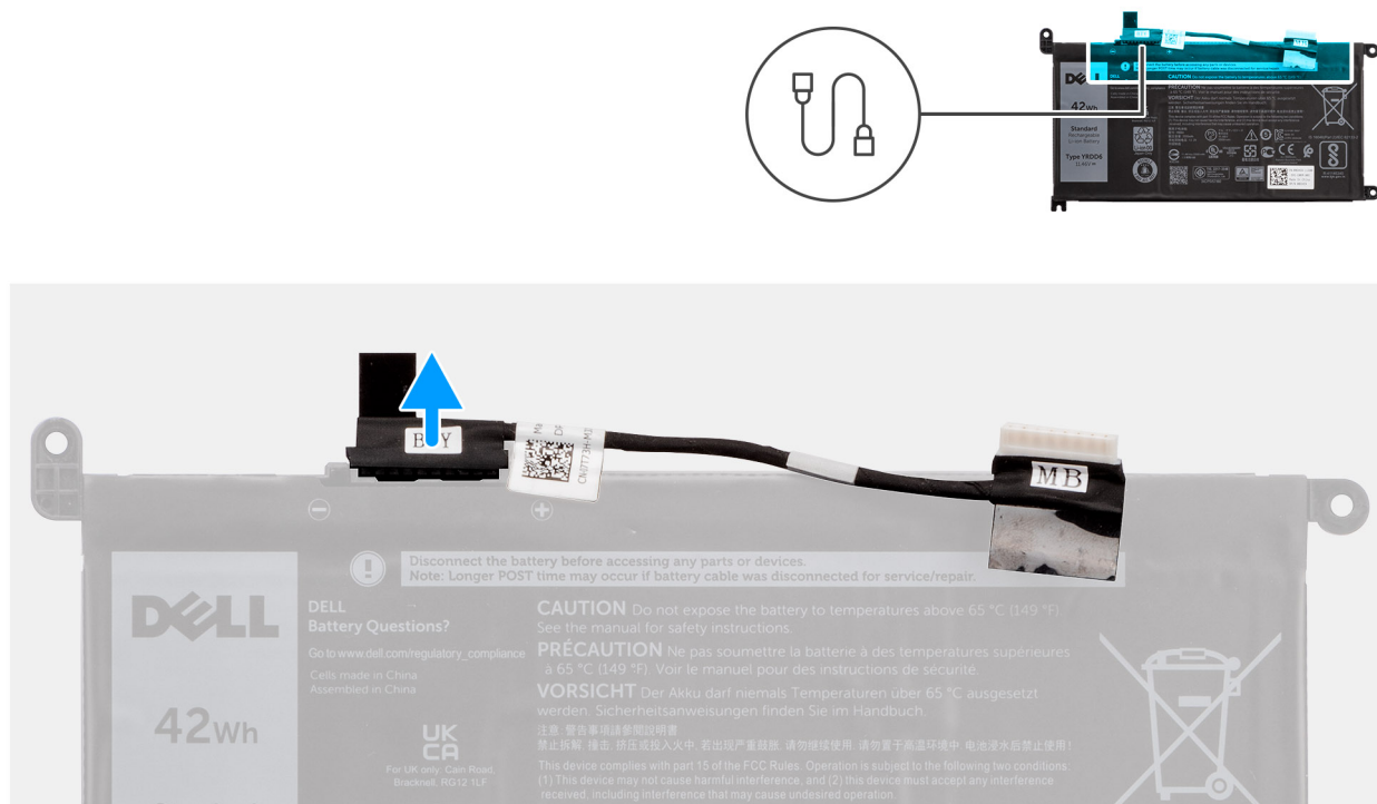
Figure 23. Removing the battery cable
