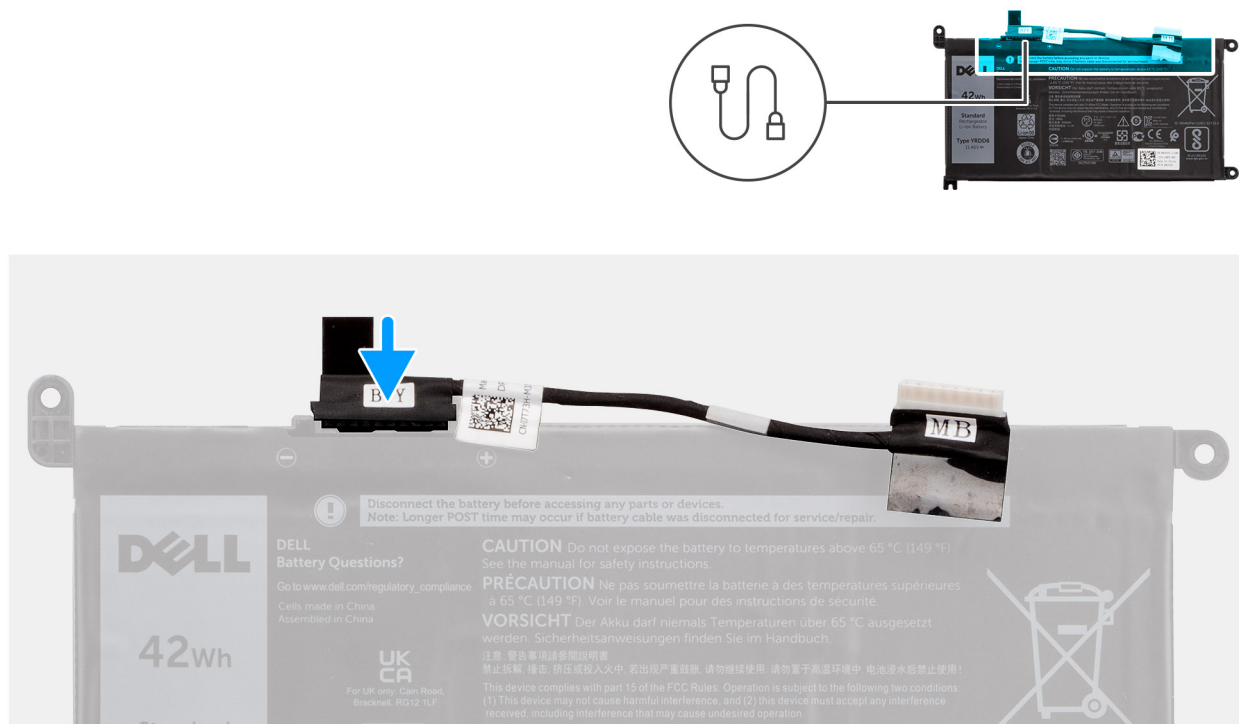
Figure 24. Installing the battery cable
