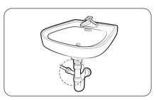
Connect the hose adapter directly to the drain pipe of the wash basin.
