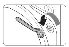
Loosen all shipping bolts on the rear of the machine using the supplied spanner.
