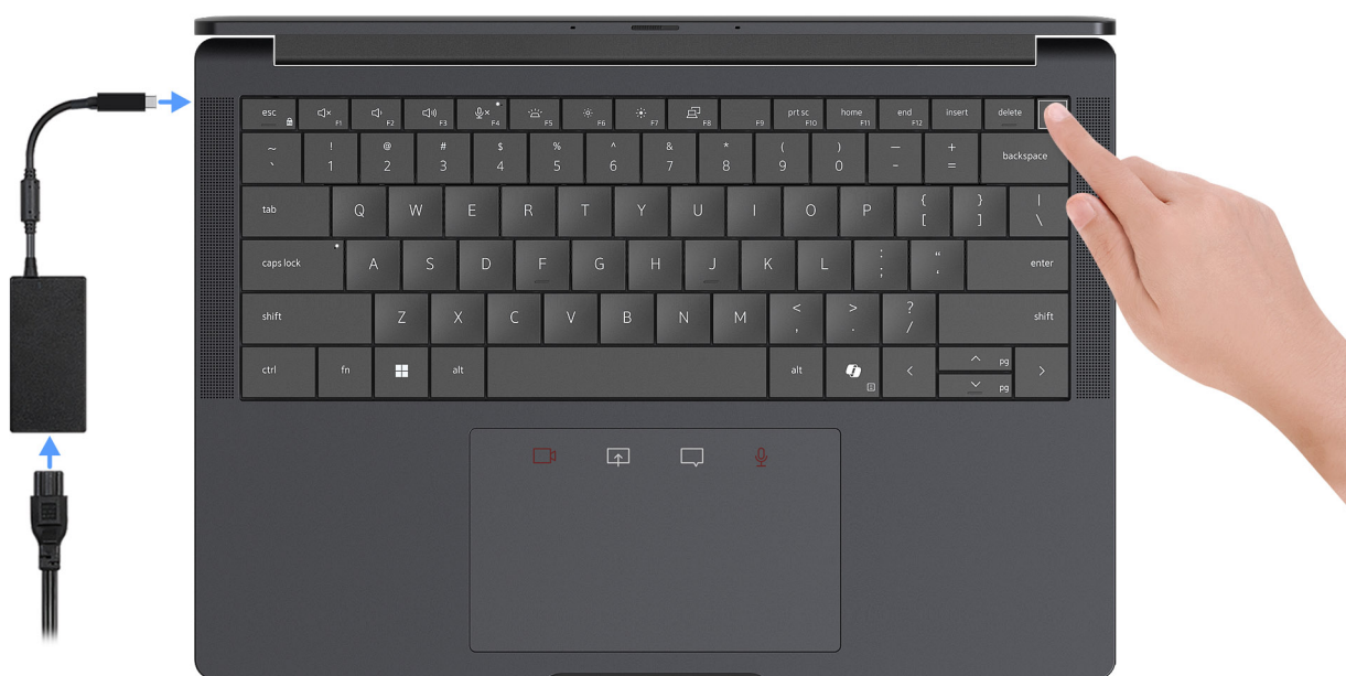
Rysunek 8. Connect the power adapter and press the power button.
