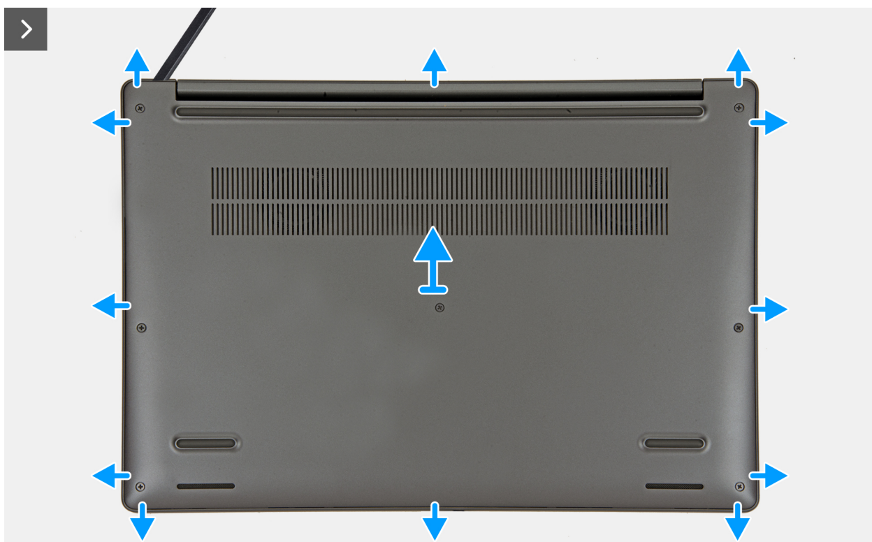
Rysunek 15. Removing the base cover
