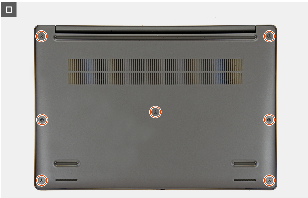
Rysunek 19. Tighten the captive screws
