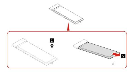
**Note:** Remove the film that covers the thermal pad (if any) when installing the M.2 solid-state drive and thermal pad.
