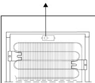
The thermostat is located on the rear wall of the cabinet (see picture above) and is controlled by the thermostat knob.
