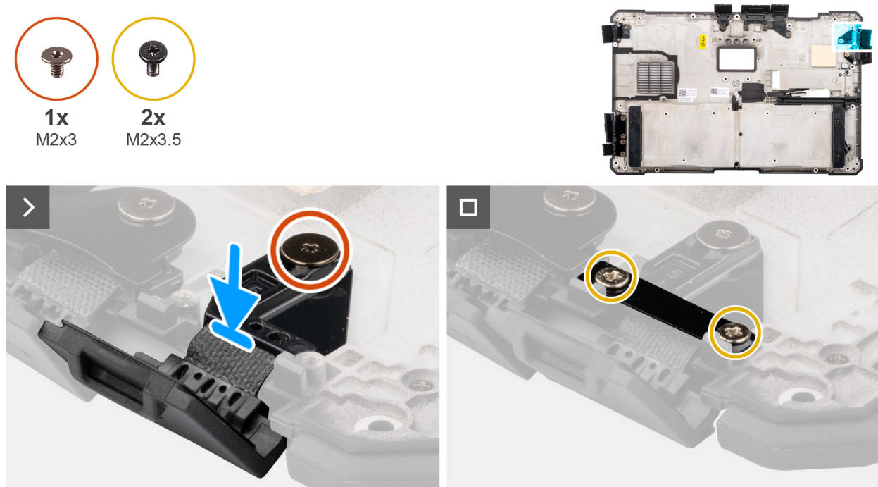
Figure 89. Installing the right Type-C port latch-door
