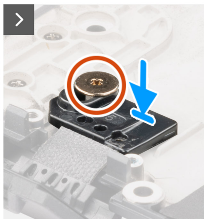
Figure 109. Installing the left Type-C port latch-door
