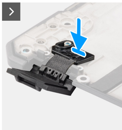
Figure 109. Installing the left Type-C port latch-door
