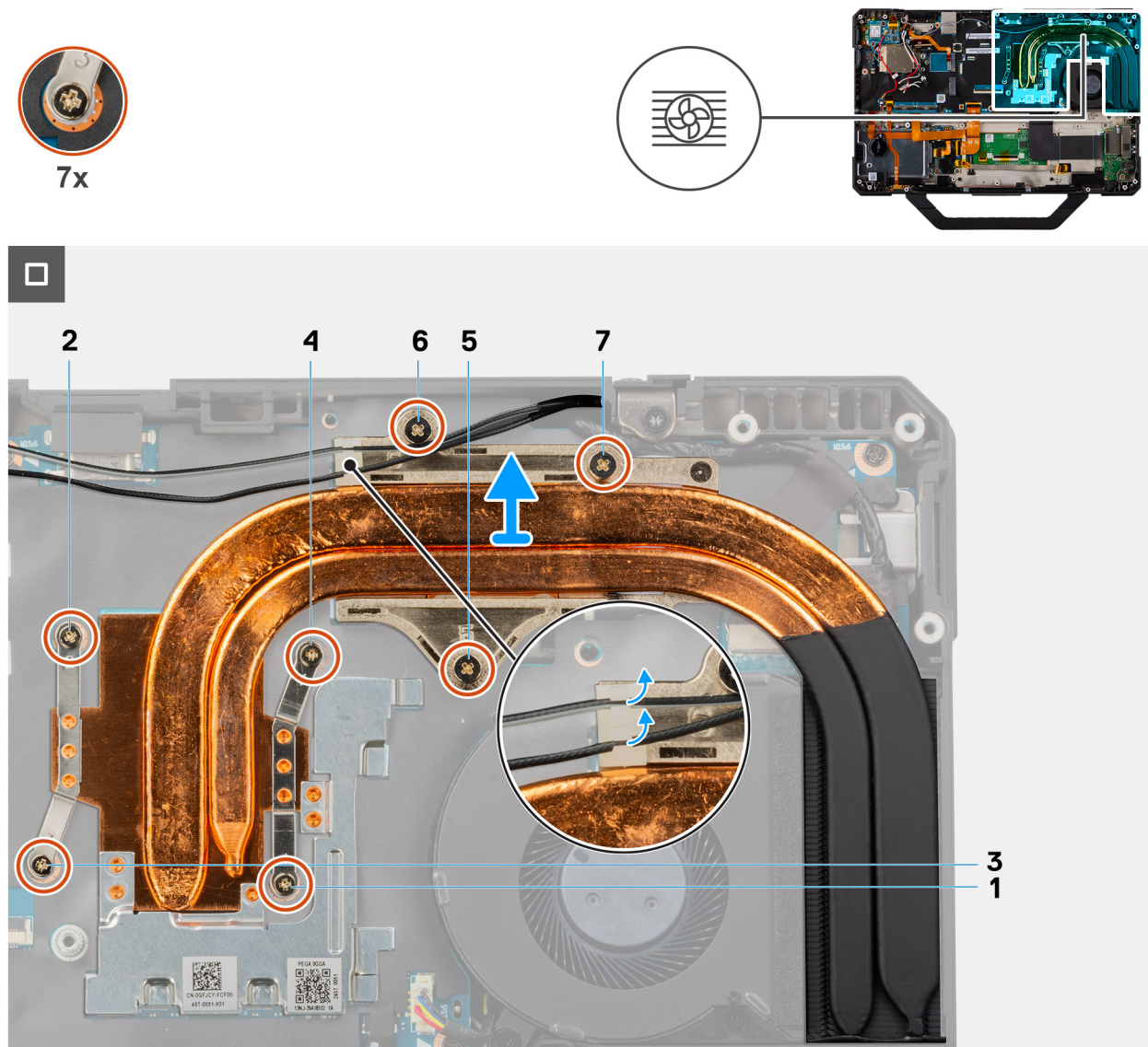
Figure 77. Removing the heat sink (for computers shipped with discrete graphics)
