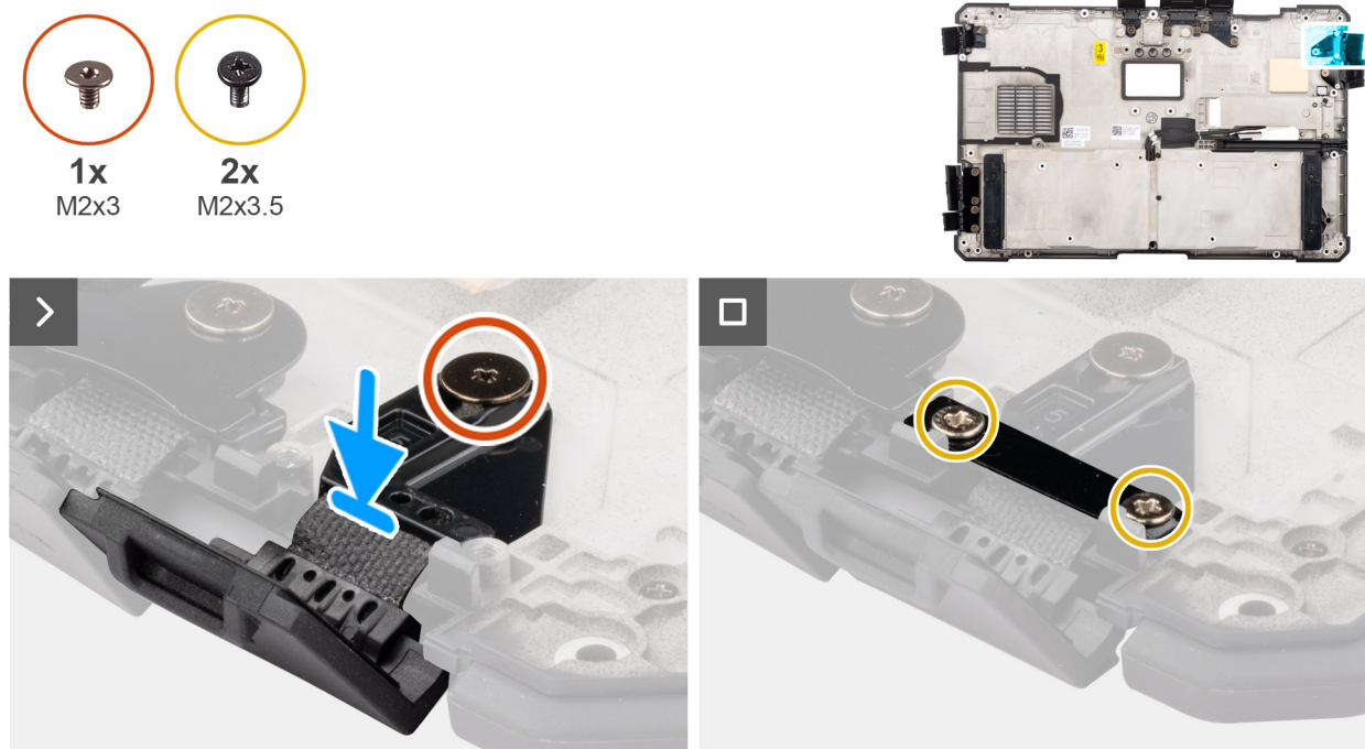
Figure 97. Installing the right Type-C port latch-door
