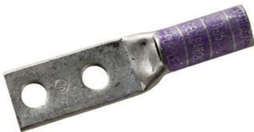
Size 6 cable, .625 inches on center between holes, 1/4 inch screw size, blue. Manufactured from electroplated tinned copper. Long barrels maximize number of crimps and are color coded. Inspection port assures full conductor insertion. 10pk.
