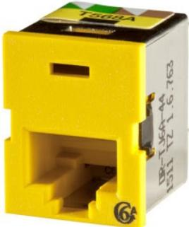
Clarity 6A TracJack, ETL verified to TIA Category 6a component specification. Front-loading and front removable. Universal T568A/B wiring label and tapered wiring towers simplify termination. Tuned to Cat6a Clarity patch cords for optimum performance
