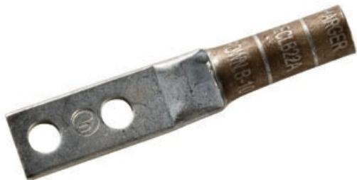
Size 6 cable, .625 inches on center between holes, 1/4 inch screw size, blue. Manufactured from electroplated tinned copper. Long barrels maximize number of crimps and are color coded. Inspection port assures full conductor insertion. 10pk.
