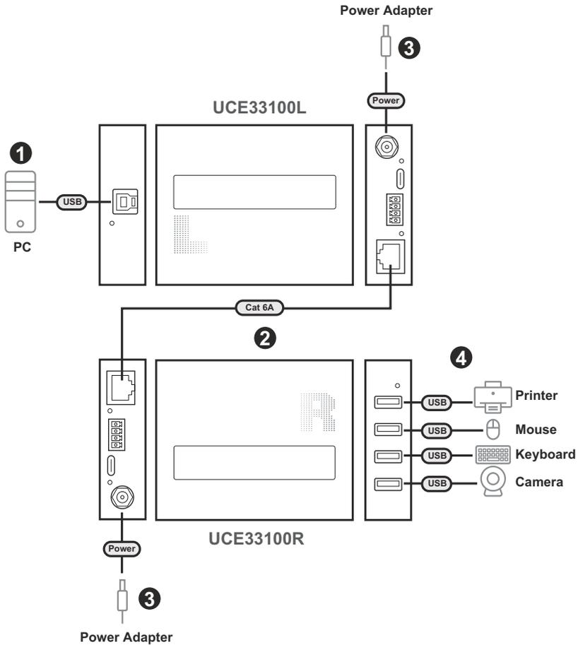
1. Connect the UCE33100L's USB Type-B port (host) to a USB port on a computer using a USB 3.2 Gen 1 cable.
