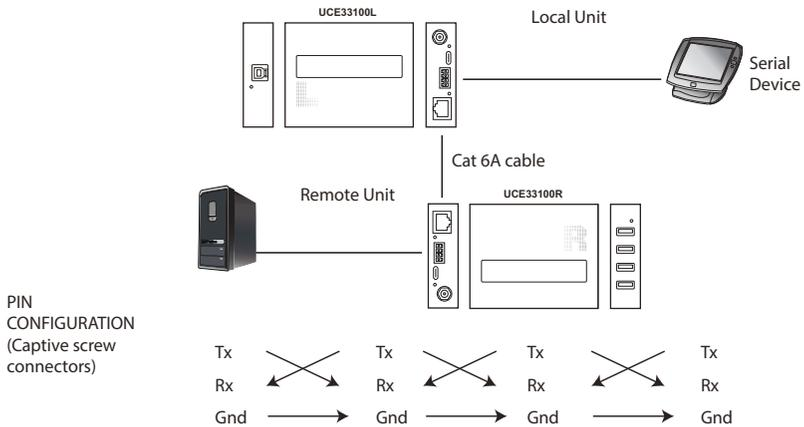
The general concept here is that a RS-232 signal can be transmitted (Tx) to the receiving (Rx) end of a unit. The received signal can then be transmitted (Tx) to the receiving (Rx) end of another unit. The RS-232 signals can be transmitted back the other way.
