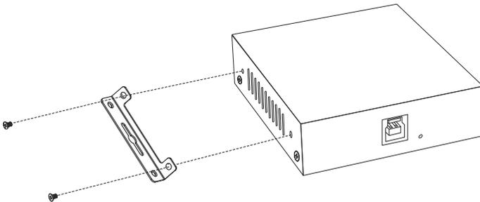
2. Through the mounting brackets, secure the unit to a selected location such as wall or ceiling using self-supplied screws.
