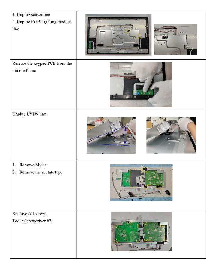
Take out PCB and Peel off all Gasket \( \) mylar \( \) Thermal pads
