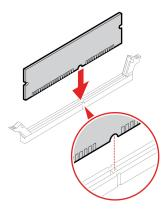
Note: During the installation, ensure that you align the memory module with the slot and press down on both ends until the latches are fully engaged with a click.
