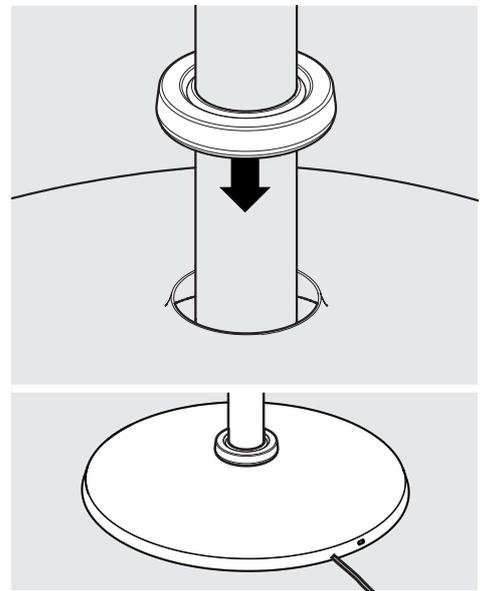
**16** With the Cover on the ground, locate and fit the Rubber Collar.
