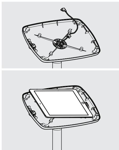
**13** Install the Tablet into the Case & connect to Power Cable.
