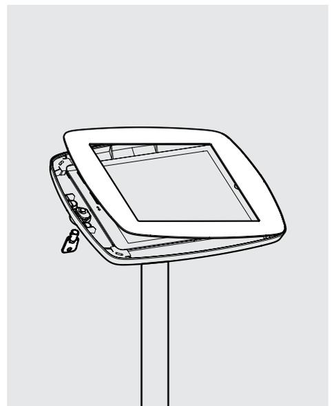
**14** Locate and lock the Faceplate onto the Case.
