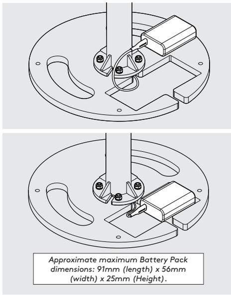
**15.2** If installing a Battery Pack, connect the Tablet's Power Cable & locate into the Base.
