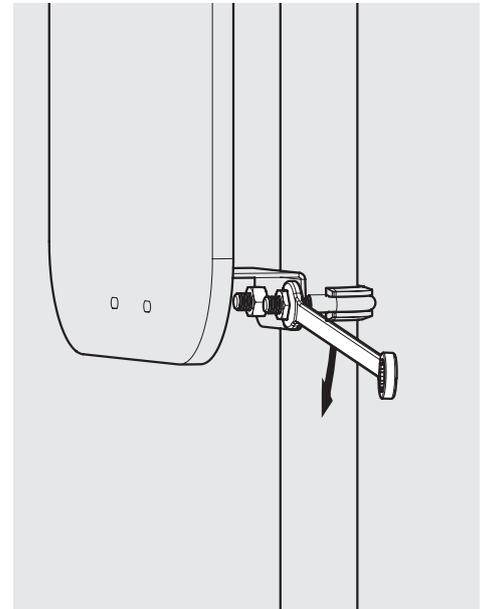
**B6** Locate & secure the bottom Bracket Mount & Mount Bolt. Tighten the nuts evenly.
