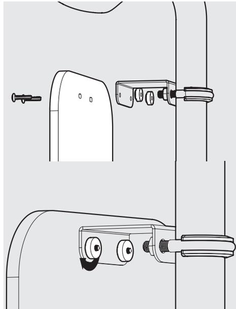
**B5** Locate the Front Board to the Bracket Mount. Secure with the supplied Plastic Screws & Nuts.
