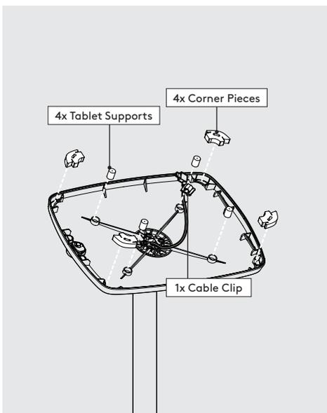
**12** Install the Tablet Setup Kit. Each kit is specific per Tablet & Case.
