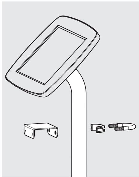
**B2** Locate the top Bracket Mount & Mount Bolt to the Floorstanding pole.
