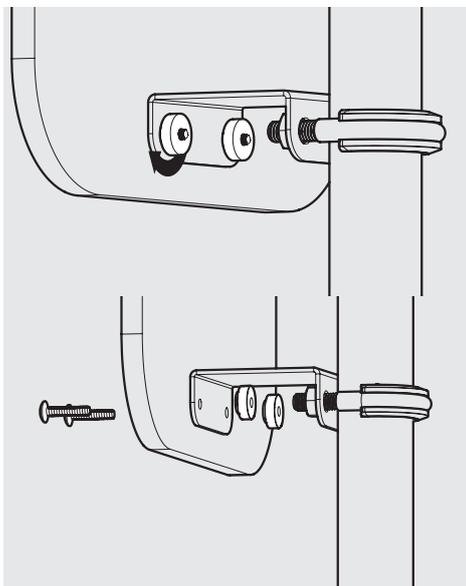
**B7** Secure the bottom section of the Front Board with the Plastic Screws & Nuts. Installation now complete.
