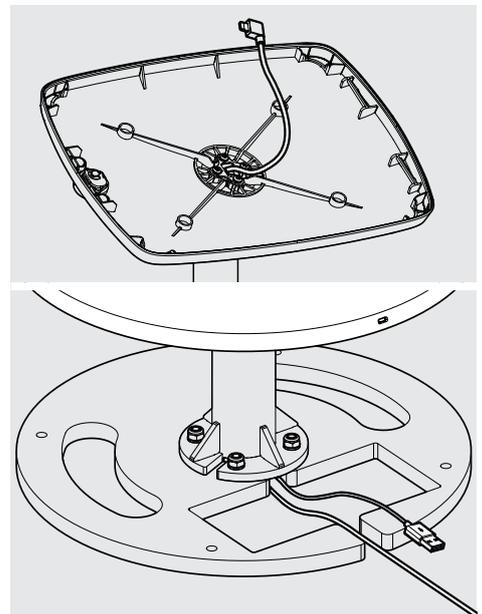
**11** Feed the Tablet's Power Cable through the Case & Floorstanding Pole.
