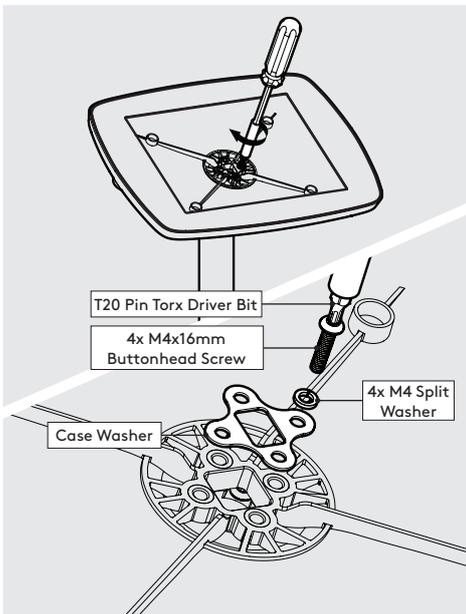
**9** Locate & secure the Case onto the Floorstanding Pole as shown. Tighten by hand.
