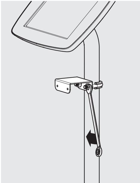
**B4** Secure the Bracket Mount & Mount Bolt to the Floorstanding Pole with the supplied Nuts. Tighten evenly.
