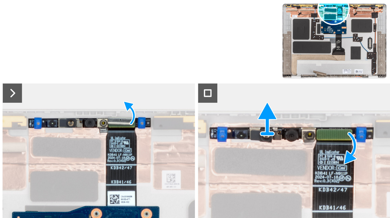
Figure 77. Removing the MIPI camera
