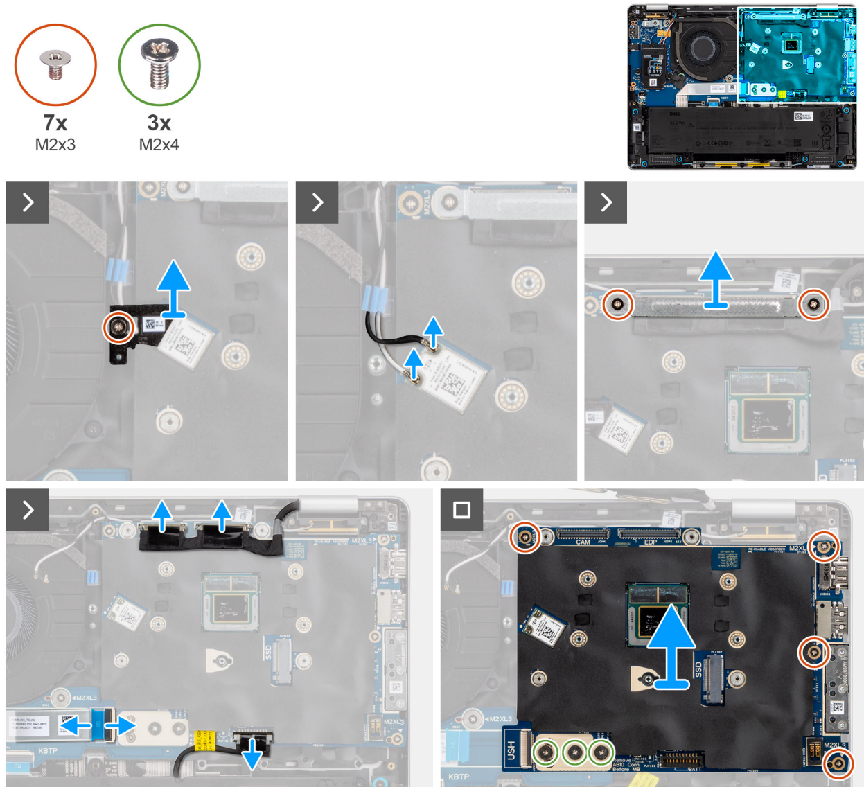
Figure 48. Removing the system board
