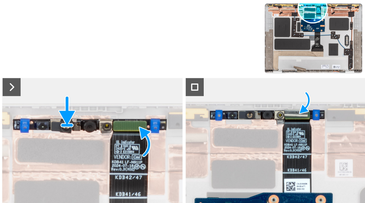
Figure 78. Installing the MIPI camera
