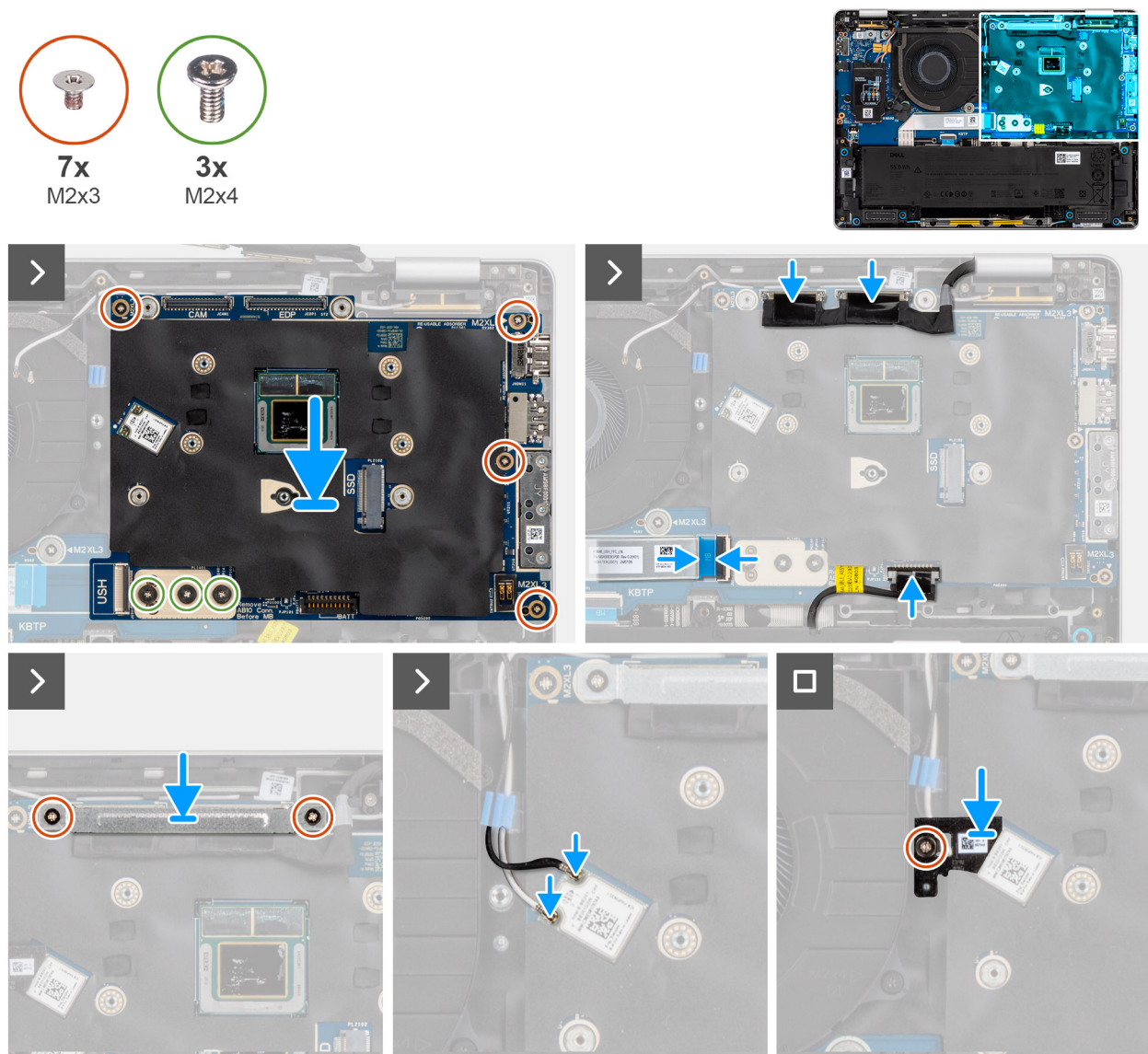
Figure 50. Installing the system board
