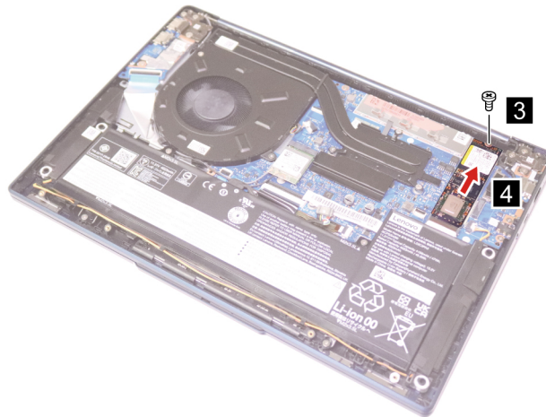
Figure 12. Remove the 2280 solid-state drive
