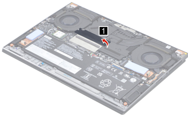
Figure 14. Peel off the memory module mylar
