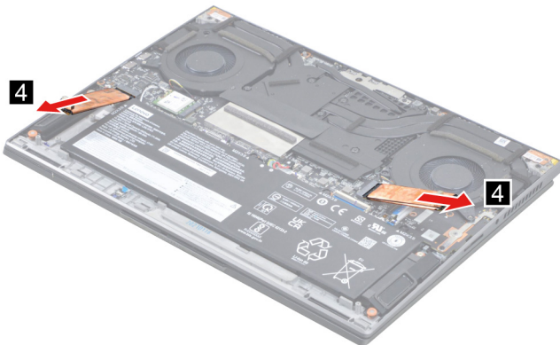
Figure 8. Remove the SSD module by pulling it away from the slot
