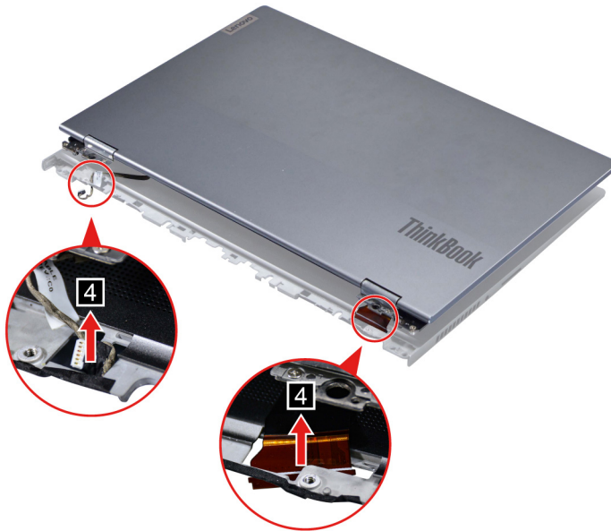
Figure 41. Remove the LCD module
