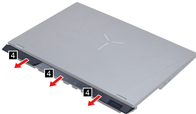
Figure 29. Turn over the computer and then remove the strip cover
