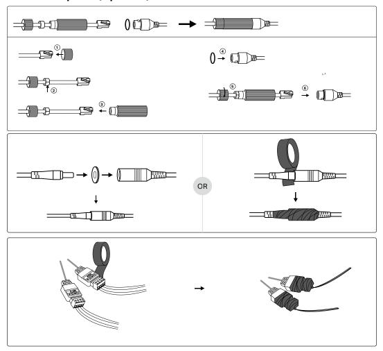
**Note:** It is recommended to waterproof the alarm/audio interface even if no alarm/audio equipment is connected.
