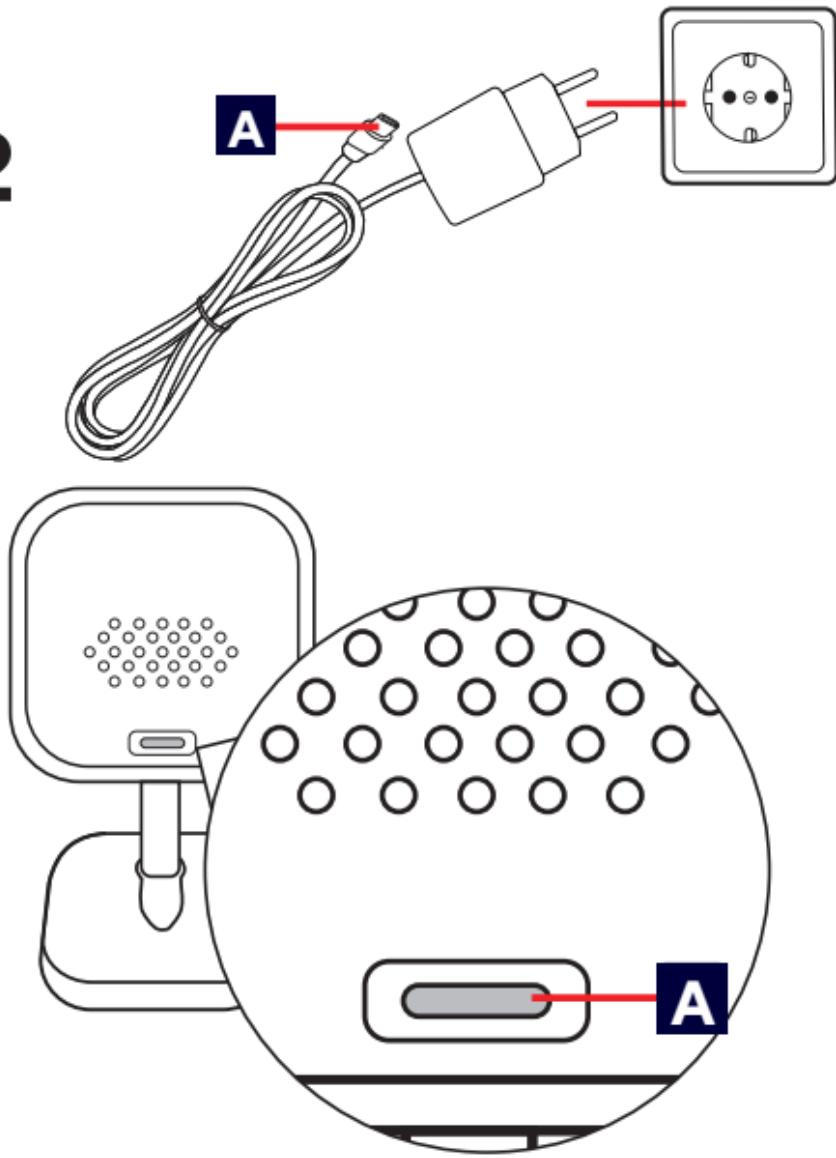
Connect the supplied USB-C power cable to the back of the camera
