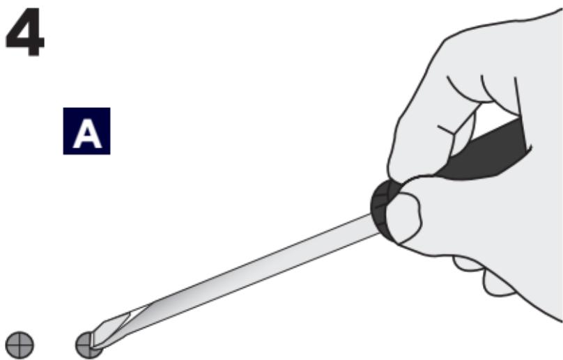
Secure the screws on a flat surface using the supplied wall plugs and screws.
