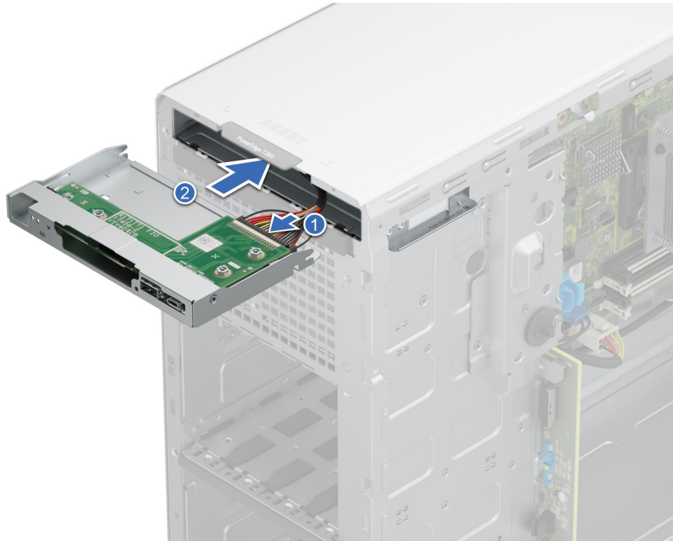
Figure 96. Installing the control panel cage
