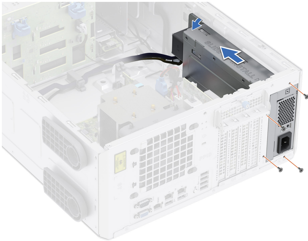
Figure 80. Removing the PSU cage
