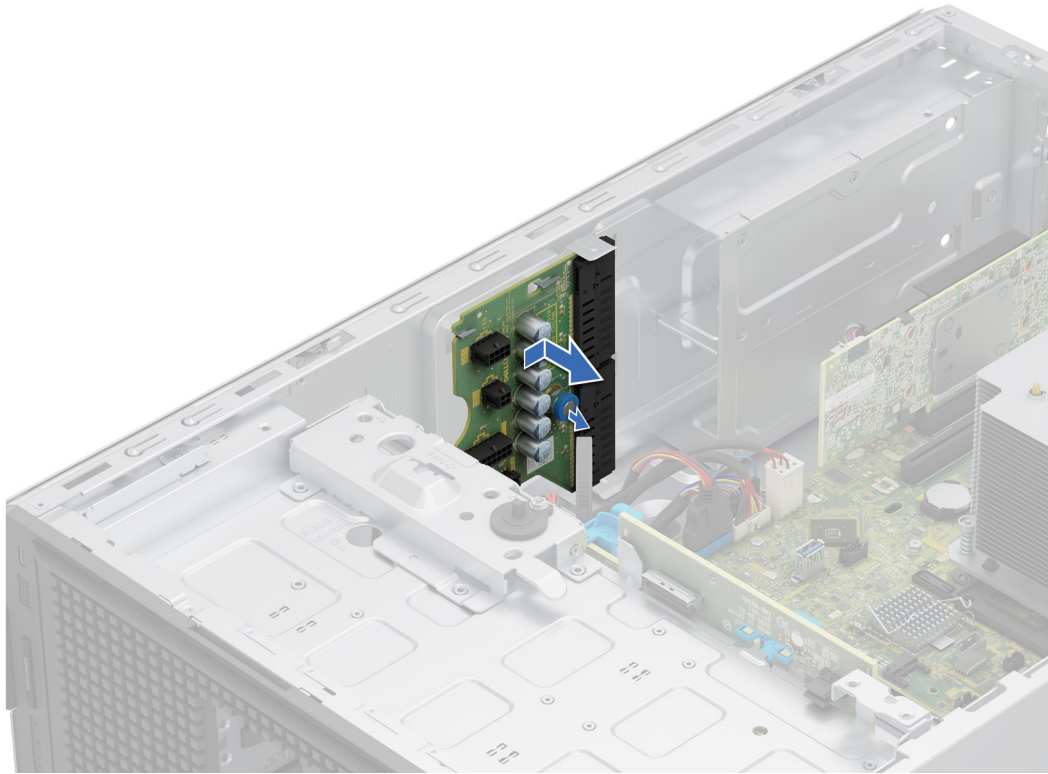
Figure 84. Removing the power interposer board
