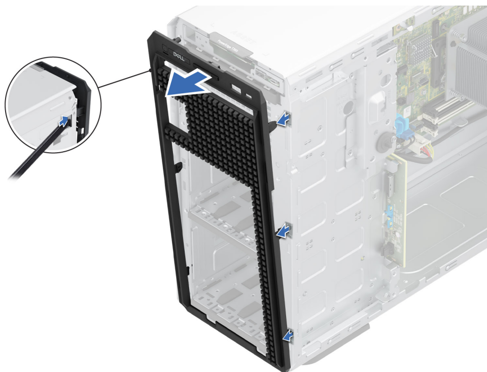
Figure 92. Removing the front faceplate
