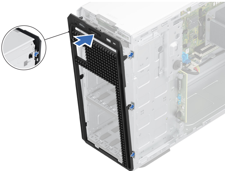
Figure 97. Installing the front faceplate
