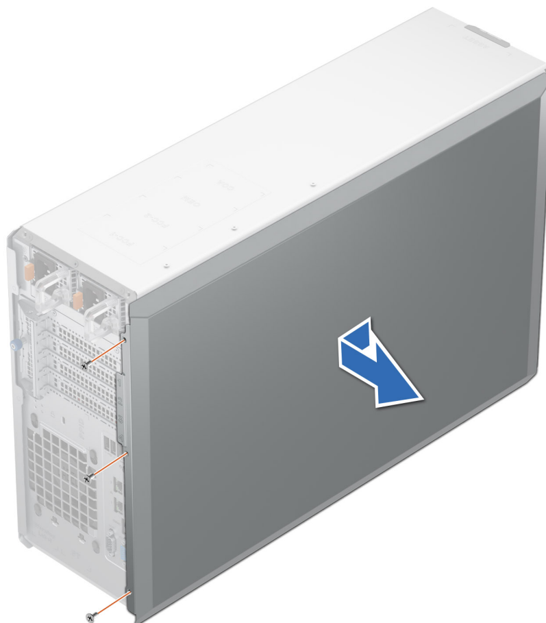
Figure 91. Removing the system side cover
