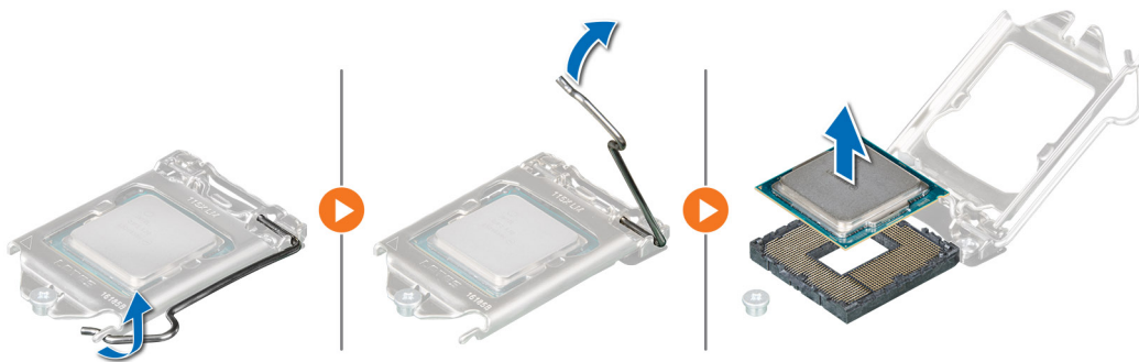
Figure 53. Removing the processor
