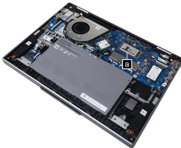
Figure 3. Area(s) on the system board where thermal interface materials are applied
