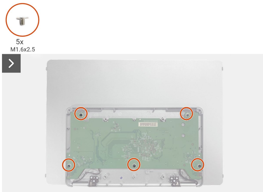
Figure 6. Removing the main board
