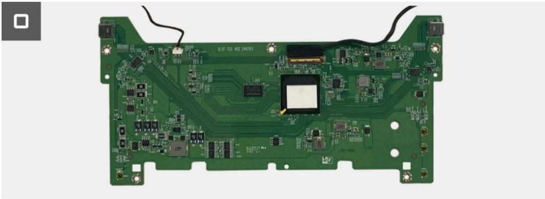
**Figura 8. Remover a placa principal**
