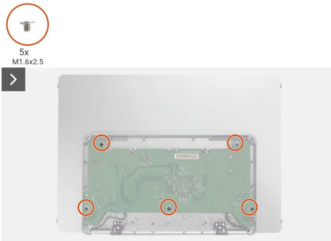
**Figura 6.** Remover a placa principal
