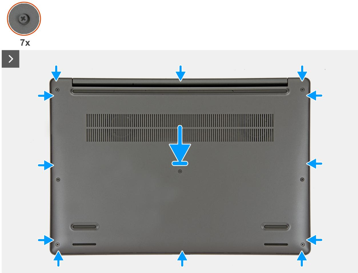
Figura 18. Installing the base cover
