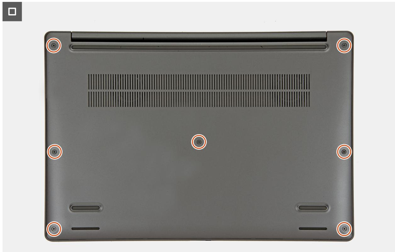
**Figura 19. Tighten the captive screws**
