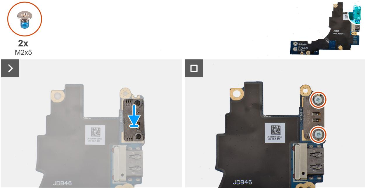
**Figura 54. Installing the left USB Type-C module**
