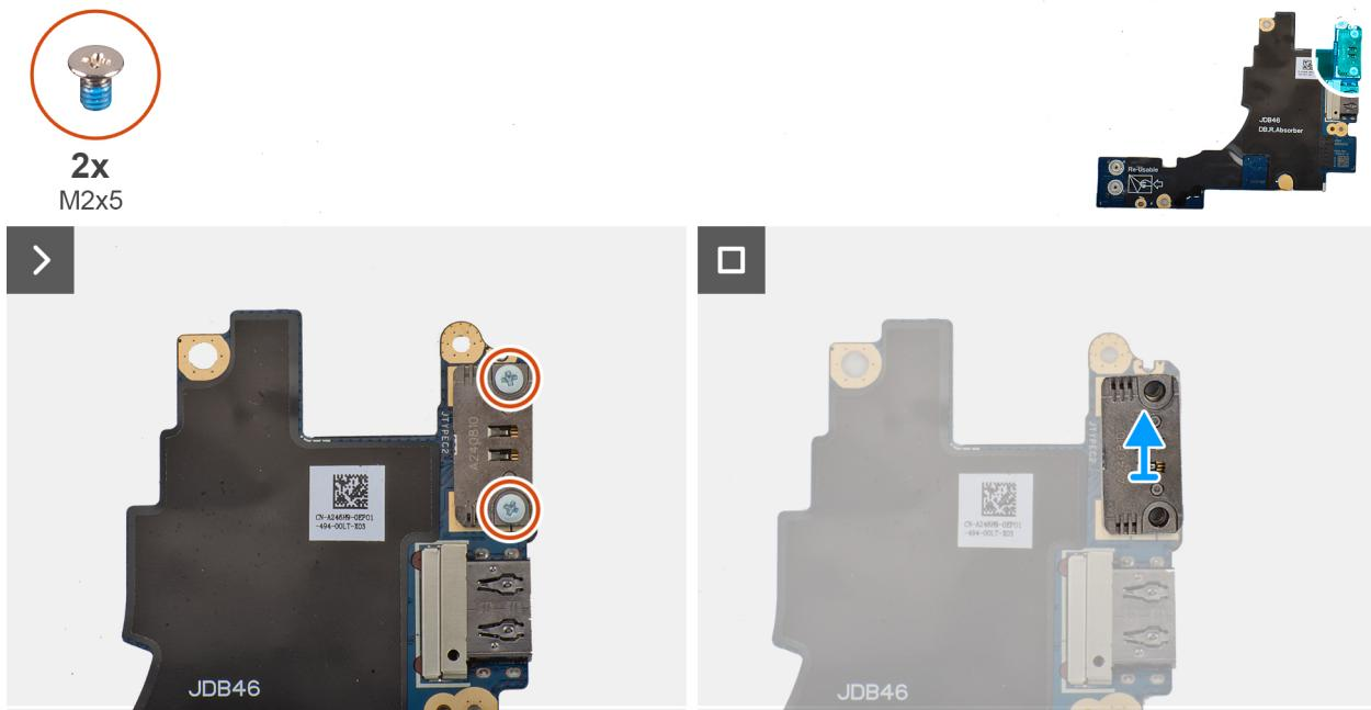
**Figura 53. Removing the left USB Type-C module**
