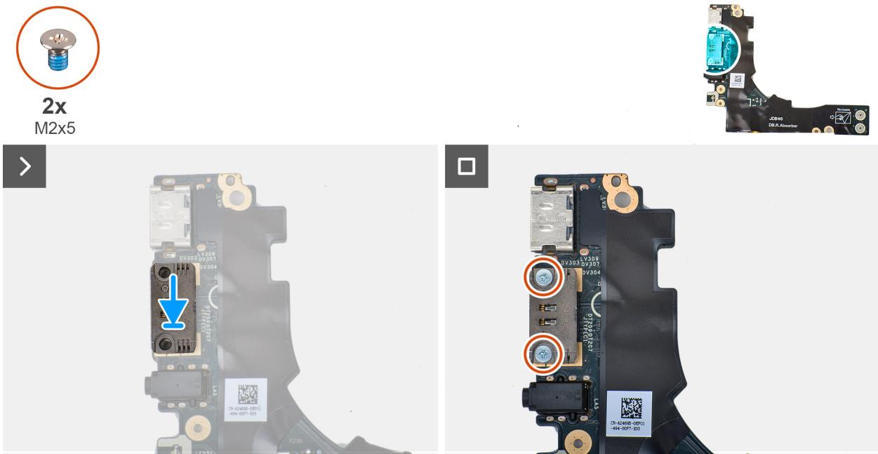
**Figura 55. Removing the right USB Type-C module**
