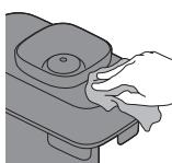
Clean the inside of the bean container and the outside of the machine with a damp cloth.
