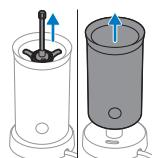
**6** Remove the whisk for cleaning after frothing.
