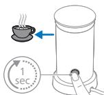
**5** Press the button for 1 second for heating and frothing milk. Press the button for 3 seconds for frothing cold milk.
