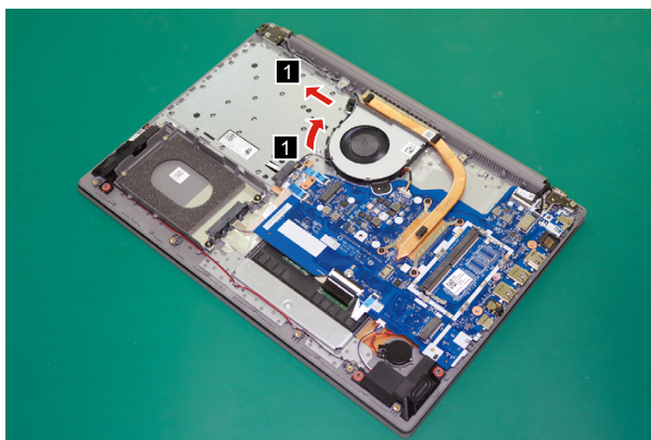
Figure 15. Release the antenna cables
