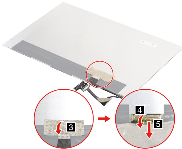
Figure 51. Remove the EDP cable
