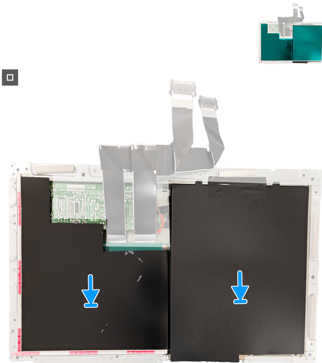
Figure 38. Installing the system board and power board
