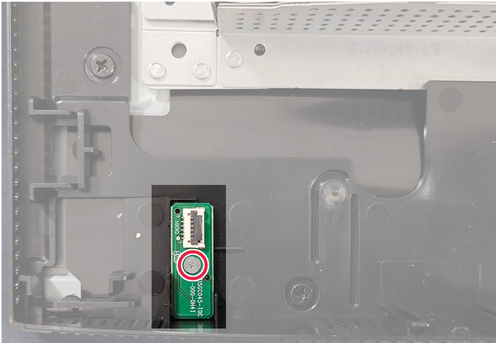
Figure 20. Removing the LENS board
