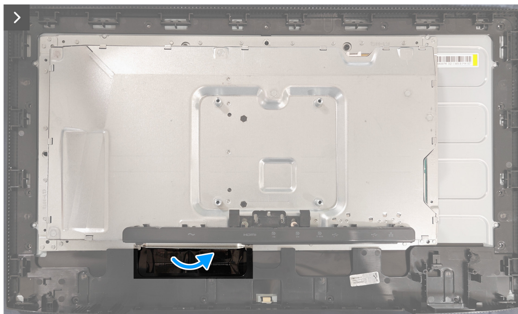
Figure 26. Removing the metal frame
