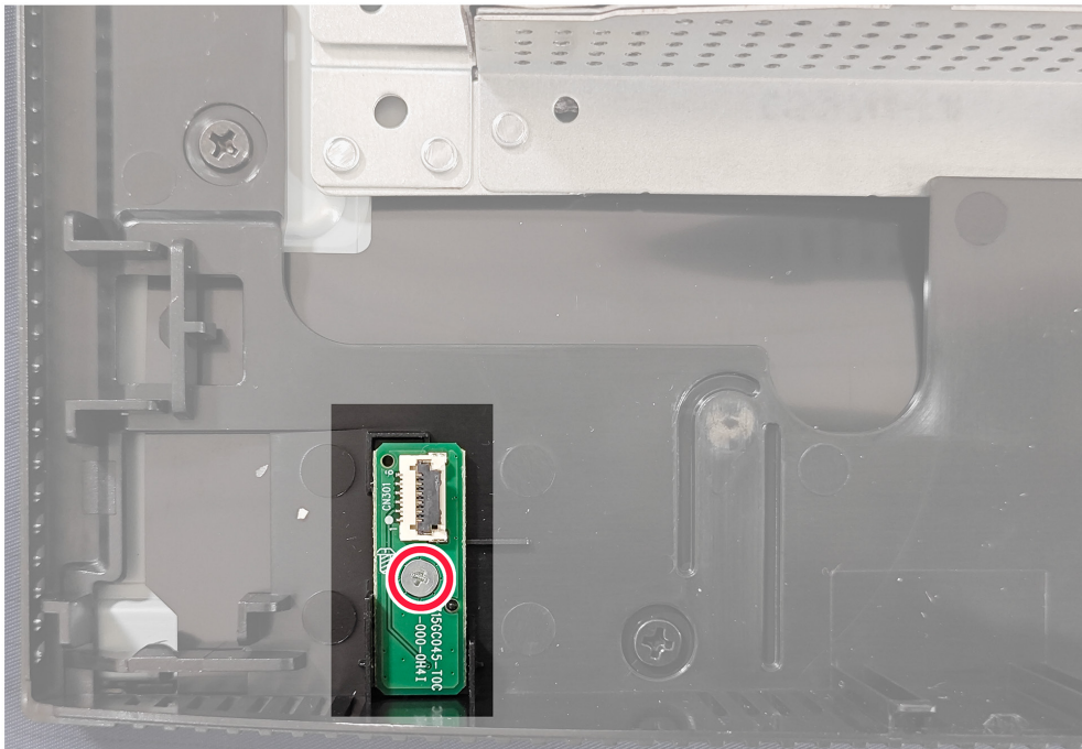
Figure 21. Installing the LENS board
