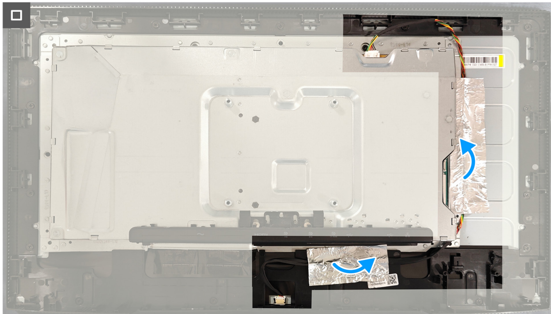
Figure 32. Installing the metal frame
