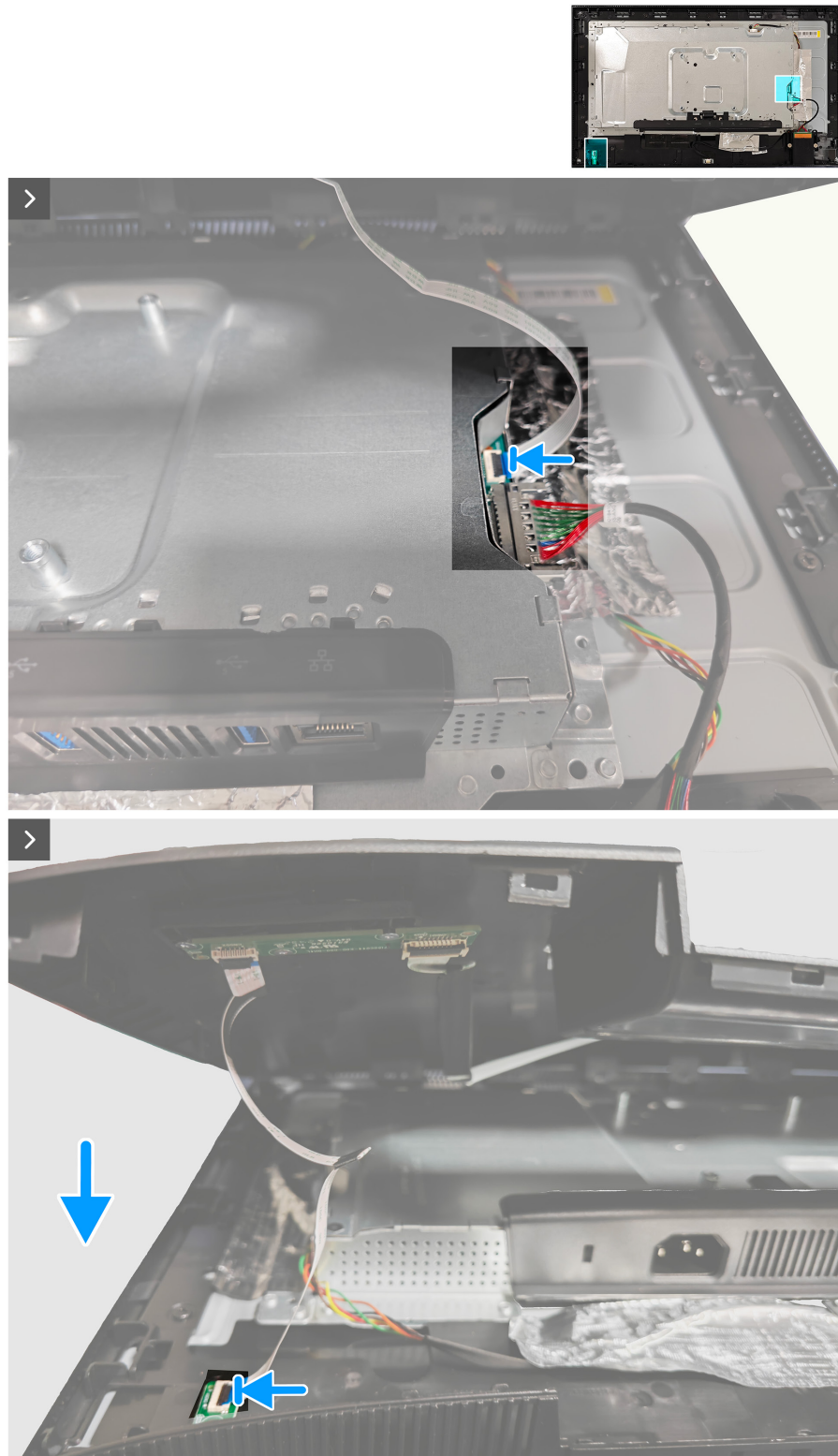
Figure 16. Installing the back cover
