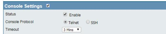
The screenshot shows the 'Console Settings' configuration page. It has a title bar with 'Console Settings' and a checkmark icon. Below the title bar, there are three settings: 'Status' with a checked checkbox and the label 'Enable', 'Console Protocol' with two radio buttons, 'Telnet' (selected) and 'SSH', and 'Timeout' with a drop-down menu showing '3 Mins'.
