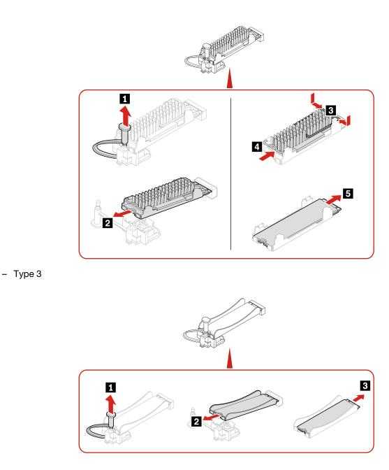
**Note:** Remove the film that covers the thermal pad (if any) when installing the M.2 solid-state drive.
