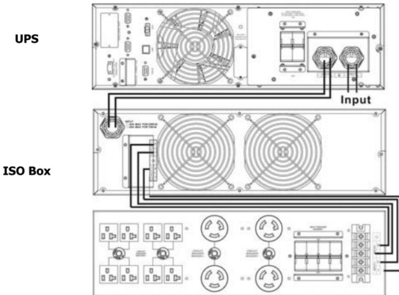
**NOTE :** Make sure that the wires are connected tightly with the terminals. Put the terminal block cover back to the rear panel.
