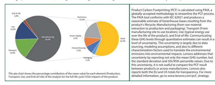
Below is a breakout of the carbon emissions of this product by both lifecycle stage (raw material extraction through product end-of-life) and greenhouse gases resulting from the manufacture of major components:
