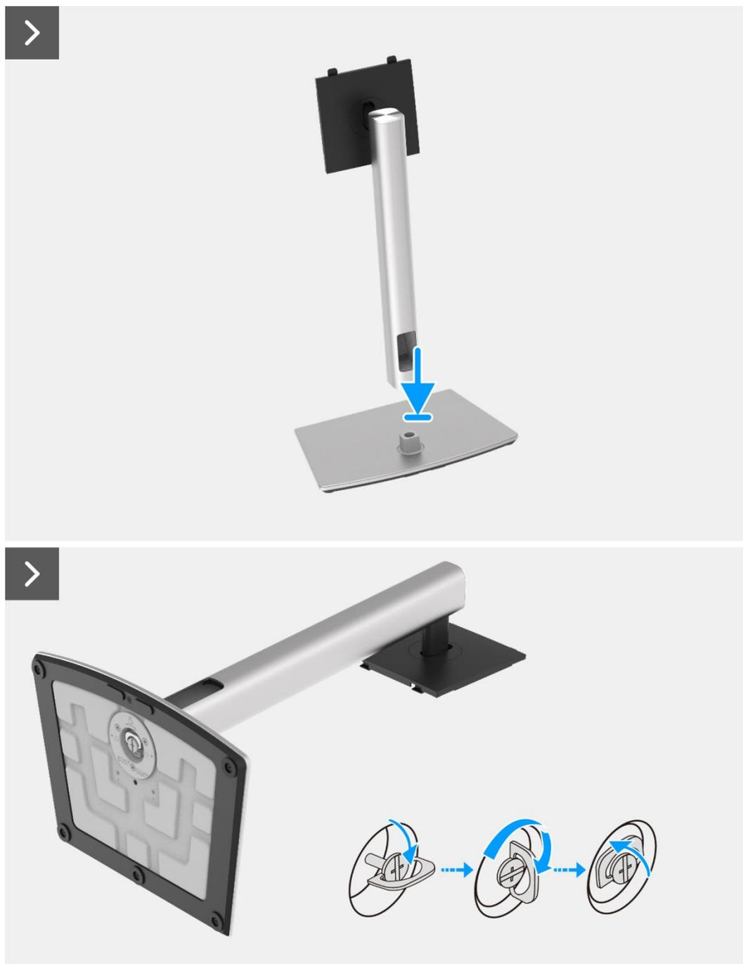
Figure 80. Installation du support
