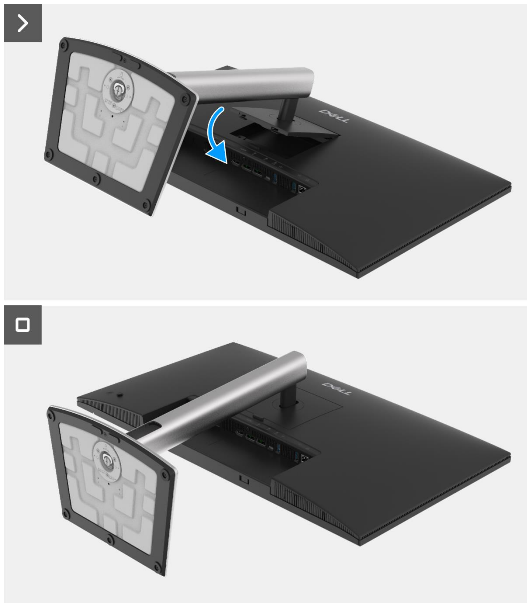
Figure 34. Installation du support
