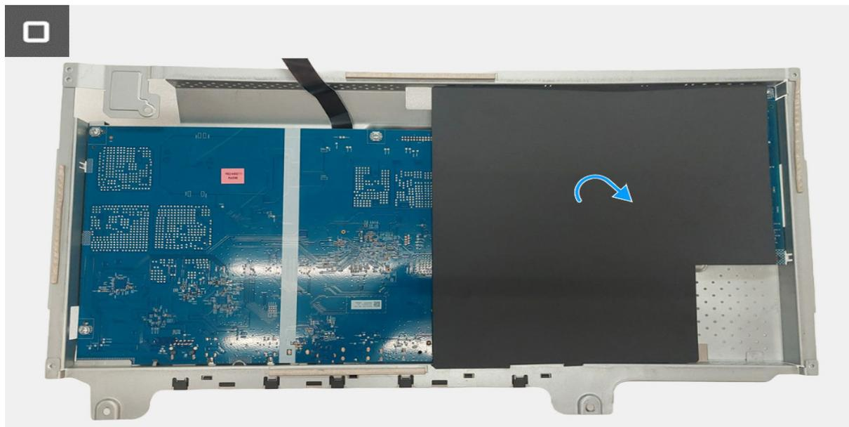
**Figura 8. Remover o chassis**
