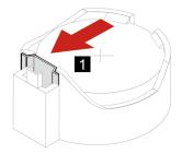
4. Remove the coin-cell battery.
