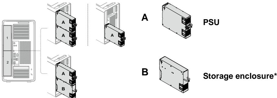
Note: PSU bay storage enclosure installation priority is higher than PSU.
