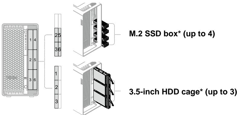
Note: M.2 SSD installation priority is higher than 3.5-inch HDD.
