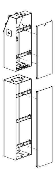
**Step 2:** Place the floor module over the six studs and tighten the 6 x M8 nuts securely.
