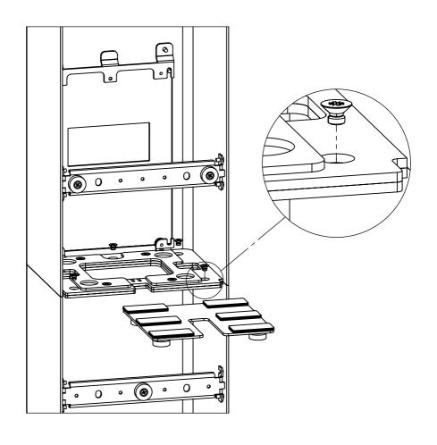
**Step 4:** Remove the protective paper from the Velcro. Position the printer as far forward as possible, and then press the printer down onto the self-adhesive Velcro.
