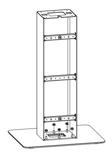
**Step 3:** Remove the printer plate by lifting it up, and then attach the top and bottom modules using the five included M5x6 countersunk screws, tightening them securely.
