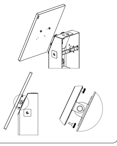
**Step 6:** To adjust the height of the screen, loosen the four screws slightly. Set the VESA mount to the desired height, and tighten the screws securely.
