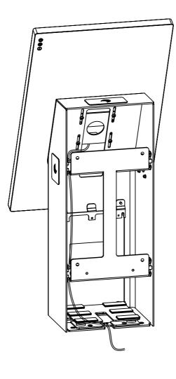
**Step 7:** Remove the protective paper from the Velcro. Guide the cables from the printer through the cable hole, position the printer as far forward as possible, and then press the printer down onto the self-adhesive Velcro.
