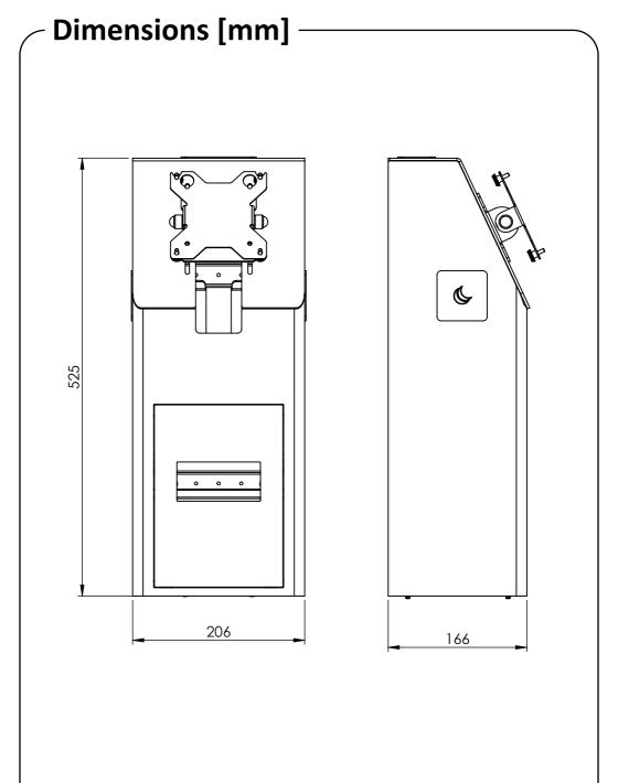
**Step 1:** Mount two of the included thumb screws to the top VESA holes on the screen and hook the screen onto the keyholes of the VESA plate. Then, attach the remaining two thumb screws to the bottom two holes on the screen and tighten them securely.
