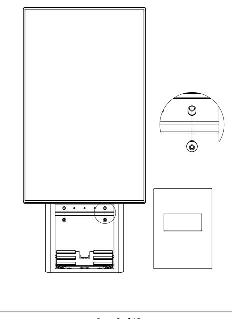
**Step 6:** Guide the cables from the screen down through the module and out through the cable hole at the bottom.
