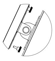
**Step 2:** To adjust the height of the screen, loosen the four screws slightly. Set the VESA mount to the desired height, and tighten the screws securely.
