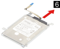
Figure 109. Remove the HDD cable
