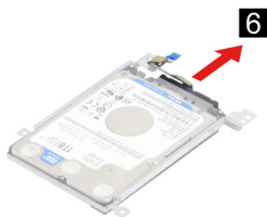
Figure 44. Remove the HDD cable
