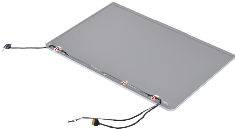
Figure 24. Release the EDP cable and camera cable
