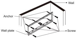
③ Hang the pre-assembled monitor unit onto the wall plate and push the bottom of the monitor to secure the brackets. To remove the monitor, simply pull down the straps to release the brackets. After assembly is complete, neatly organize all wires and cables.
