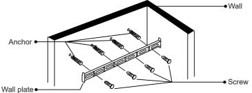
③ Hang the pre-assembled monitor unit onto the wall plate and push the bottom of the monitor to secure the brackets. To remove the monitor, simply pull down the straps to release the brackets. After assembly is complete, neatly organize all wires and cables.
