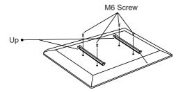
② Position the wall plate and secure it with 4pcs of ST7x55mm screws and anchors; drill holes if needed.
