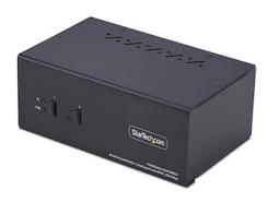
The HDMI and DisplayPort KVM switch enables a mixed-display setup of an HDMI and a DisplayPort monitor without the need for adapters or converters. It allows you to share peripherals, including a keyboard, mouse, audio device, and dual monitors, between two computers.
