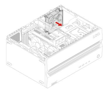
**Note:** Elongate the rubber that fixes the fan to remove the fan from the chassis.
