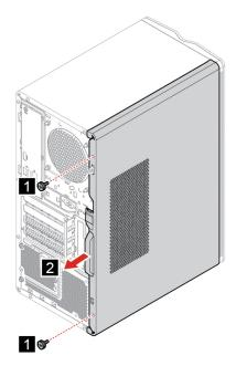
**Note:** The screw can be conveniently removed by hand without the need for any special tools.
