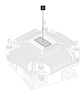
Figure 1. Illustrations of the thermal pad area
