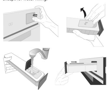
After the first filling, in case of longer cooking cycles, once water will have ran out, it could be necessary to add it again, in order to complete the cycle: the oven will prompt it in case it is needed.
