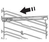
Remove the shelf guides from the oven and remove the protective plastic from the sliding runners.
